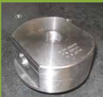
A steel scrubber-bottle cap (finished at left, and in GibbsCAM's Cut Part Rendering feature, right, for toolpath verification).
