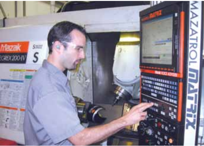
Nathan Neels makes an adjustment on a control for the 7 axis Mazak Integrex machine.
